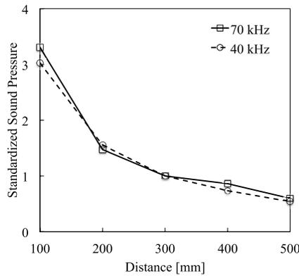
**Fig. 3.** Attenuation of sound pressure versus distance. The sound pressure level was measured in a range from 100 mm to 500 mm. The measurement data has been standardized by the value of the position of 300 mm. The peak-to-peak voltages of the sinusoidal driving signals at 70 kHz and 40 kHz were 70 V and 30 V, respectively.
