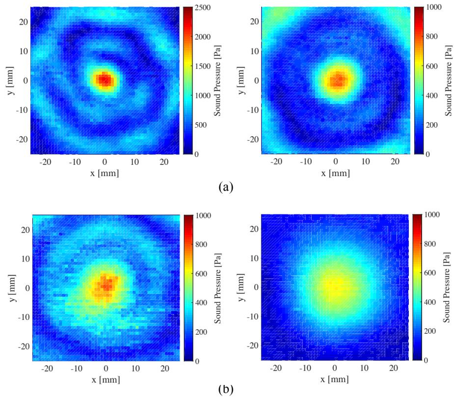
**Fig. 5.** Sound pressure distribution. Two dimensional spatial distribution of the sound pressure around the focus. Left: 70 kHz phased array. Right: 40 kHz phased array. (a) Focal length: 150 mm. (b) Focal length: 300 mm.
