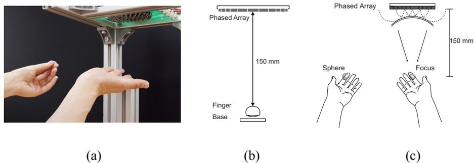
**Fig. 8.** Experimental setup for the psychophysical experiments. We have set up a base for indicating the position of the finger. When the subject places the finger on the base, finger pad and the focus were in the same position.
