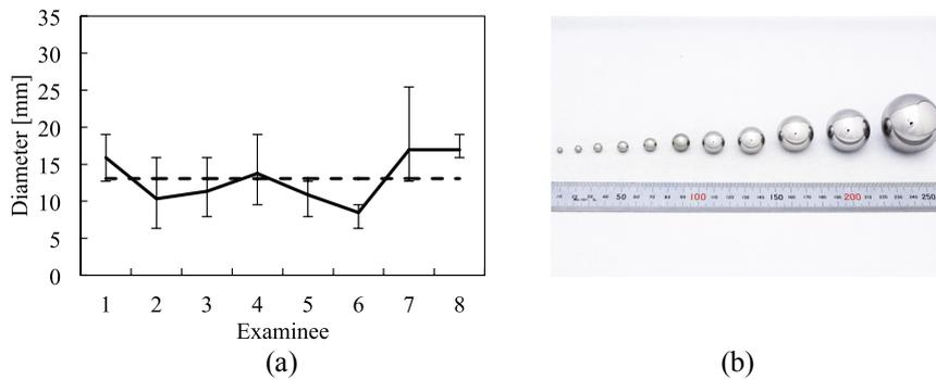
**Fig. 10.** (a) Perceived focus diameter. The mean value was 13.1 mm. (b) Photograph of the metal spheres used in the comparison test. The diameters of the spheres are 4, 5, 6.35, 7.93, 9.52, 12.7, 15.87, 19.05, 25.4, 30.16, and 41.27 mm.
