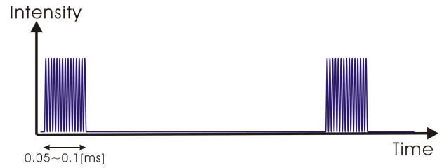
Fig. 13 Waveform for Stimulating Nerve Systems
