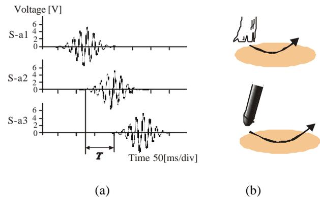
**Fig. 13:** Signal waveforms of the stimulators (a) and the image of tactile feeling (b). Subjects felt something to sweep over the finger. Perception of the associated object changed according to the carrier frequency and the amplitude.
