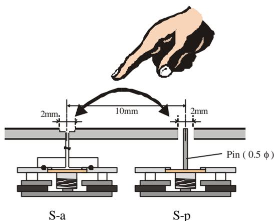
**Fig. 10:** Set up of air-pin discrimination test in Experiment II .
