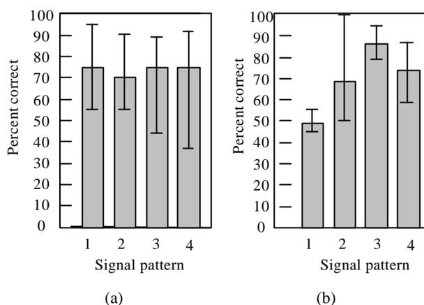
**Fig. 11:** Correct answer ratio of the air-pin discrimination test for fingerchip (a) and thenar (b), for signal patterns 1) sinusoidal wave of 20Hz, 2) sinusoidal wave of 100Hz, 3) random phase signal and 4) pulse sequence.
