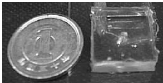
Fig. 10: Sensing and powering coils in silicon rubber.
