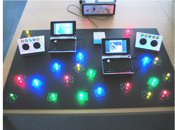
Figure 1. A demonstration of Two-Dimensional Communication (2DC) technology. A black sheet is the 2DST sheet. A box above the sheet is a microwave oscillator. It applies 10 watts of power into the sheet. LEDs, speakers, and fans work using the power transmitted through the sheet. Two PCs communicate with each other. The PC on the right is reading movie data from the hard drive of the PC on the left and displaying it. All devices are just touching the sheet. They can work anywhere on the sheet without any direct connection.
