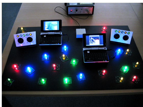
Fig. 1 A demonstration of Two-Dimensional Communication is shown. In this demonstration, we have two PCs rigged with our special couplers placed on the 2D Communication sheet. The PC on the right is reading a movie file from the hard drive of the PC on the left wirelessly through the sheet. In addition, LEDs, fans and speakers acquire electricity from the sheet. Data transmission and powering are both realized wirelessly through the sheet.
