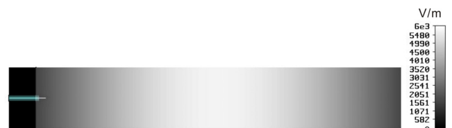
Fig. 4 Average amplitude of the electric field in the sheet at 2.4 GHz. The sides are the node and the center is the anti-node for the electric field.
