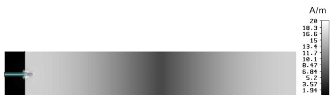
Fig. 5 Average amplitude of the magnetic field in the sheet at 2.4 GHz. The sides are the anti-node and the center is the node for the magnetic field.
