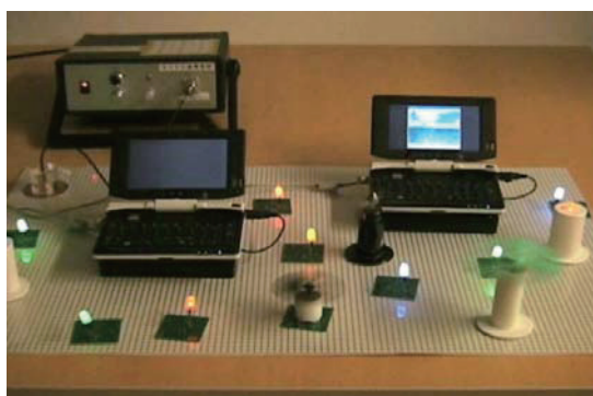
Fig. 1 The demonstration of both signal transmission and power supply through the Two-Dimensional Communication sheet. The right PC displays the movie data sent from the left one. The LEDs and the small fans receive electricity from the power source shown in the upper-left of the picture via the 2DC sheet.
