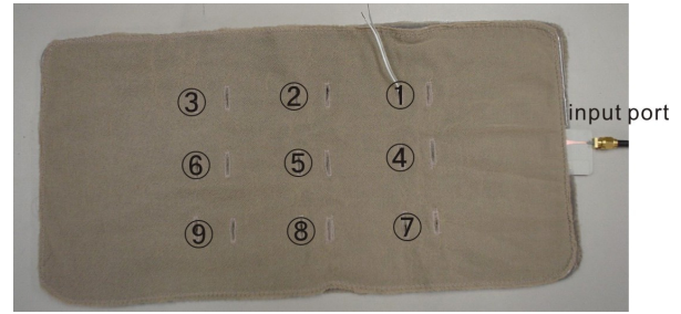
Fig.8 Textile 2DC sheet. Each number denotes the position.
