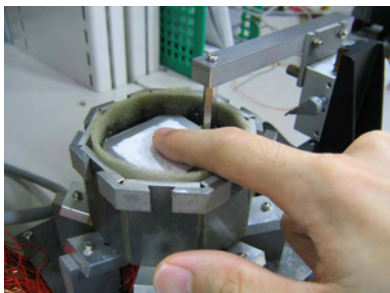
Fig. 8 A photograph of the display in use. The ultrasound reflective film is put just on the surface of the water.
