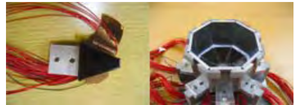
Fig. 5 Linear arrays used in the prototype system. Left: One unit of the linear array. Right: Linear arrays arranged at the edge of the octagon. Each linear array is fixed at the bottom of the water bath.
